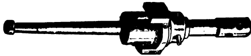
FIG. 130.—The Dudgeon Boiler Flue Expander, as used for making expanded joints on the flues of large boilers.
